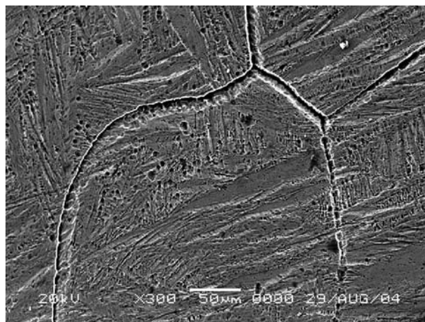
Fig. 2 SEM micrograph of martensite plate in Fe–24.5%Ni–4.5%Si alloy, austenitized at 1100 °C for 45 h
