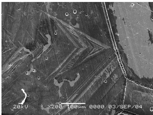
Fig. 1 SEM micrograph of martensite plate in Fe–24.5%Ni–4.5%Si alloy, austenitized at 1100 °C for 24 h
